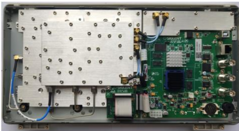
Figure 4-4 View of front panel subassembly with the mainboard
