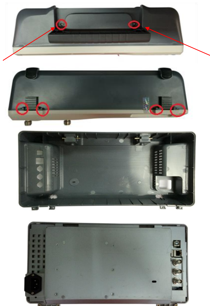
Figure 4-1 Removing the Rear Panel Screws
